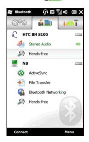
The double arrowhead ( ) that is displayed to the right of a service indicates that the service is connected with your headset. If you turn off your headset, the double arrowhead disappears to indicate that the service has been disconnected. Next time you turn on and use your headset again, you need to manually reconnect each service. Tap a service and then tap *Connect*.
